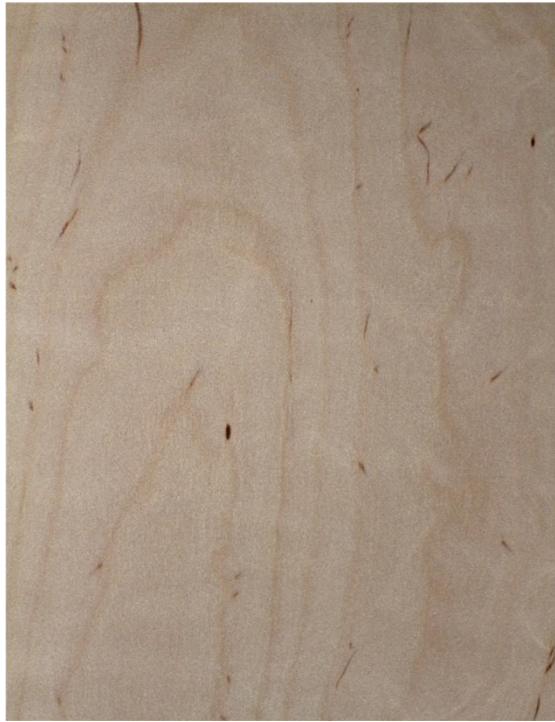
BR: colour defects, flames and curly figuring, some knots max \varnothing 8 mm
