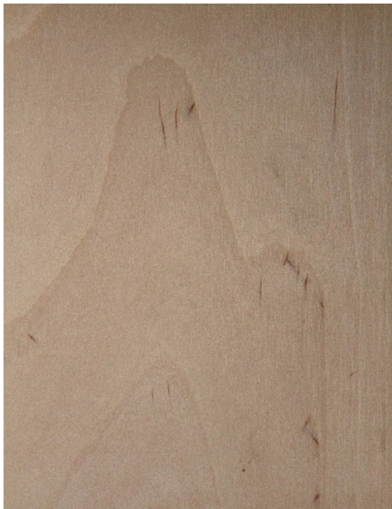
BR: colour defects, flames and curly figuring, some knots max \varnothing 8 mm
