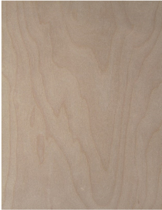
AB: small color defects, flames and curly figuring / small streak and overlaps
