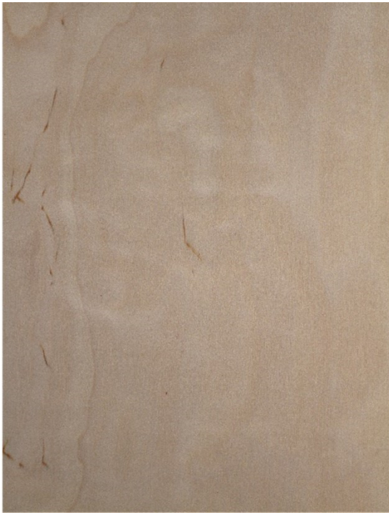
B: colour variation, flames and curly figuring / some knots or knotholes max Ø7-8 mm
