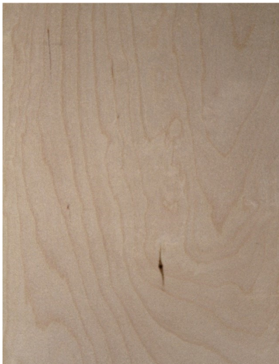
AB solid knots max \varnothing 5 mm / deviation of the grain
