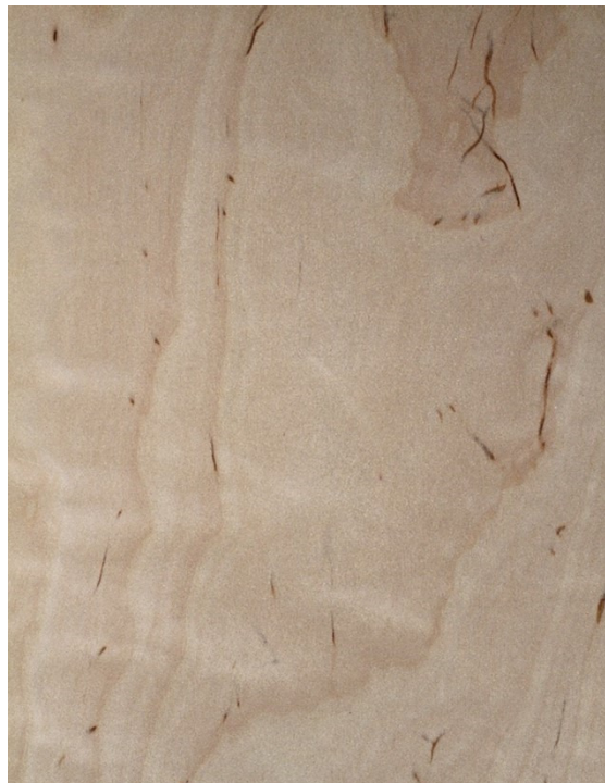
BR: colour defects, flames and curly figuring, some knots max \varnothing 8 mm
