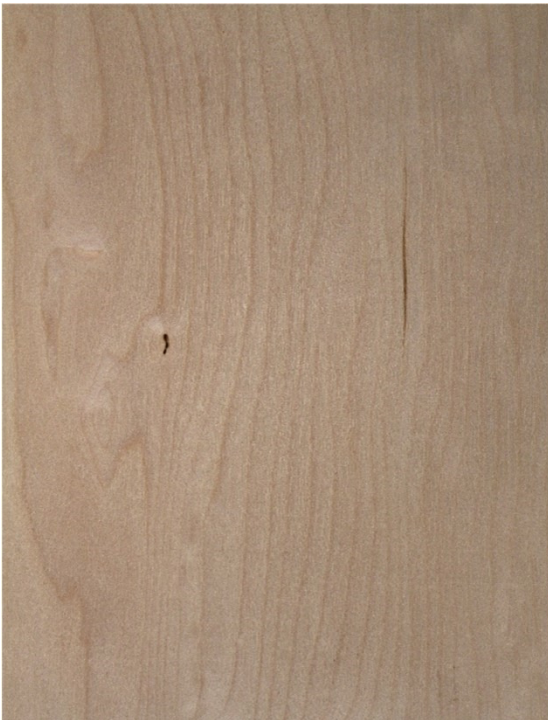
B: small streak and overlaps / deviation of the grain
