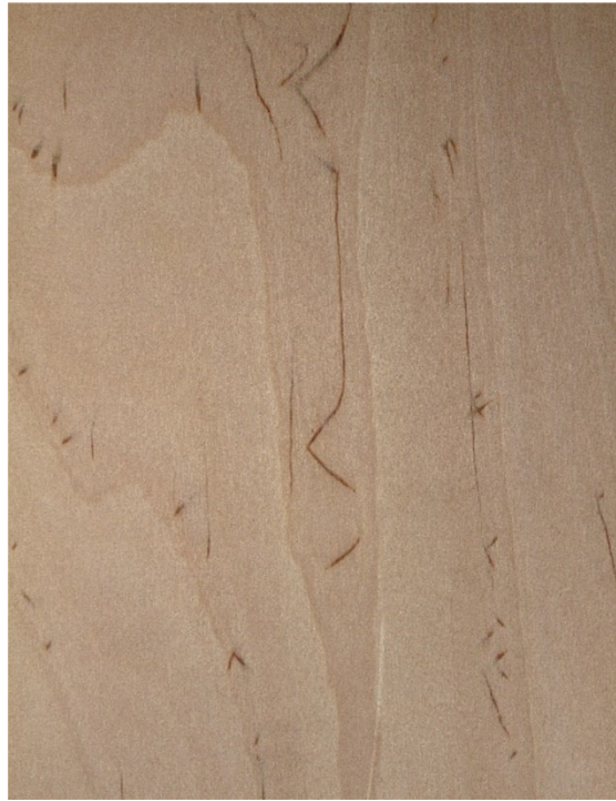
BR: colour defects, flames and curly figuring, some knots max \varnothing 8 mm
