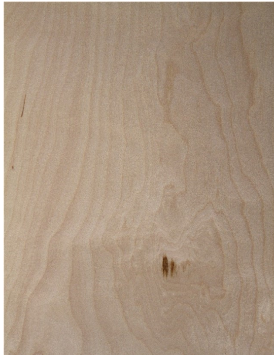
B: colour variation, flames and curly figuring / some knots or knotholes max Ø7-8 mm
